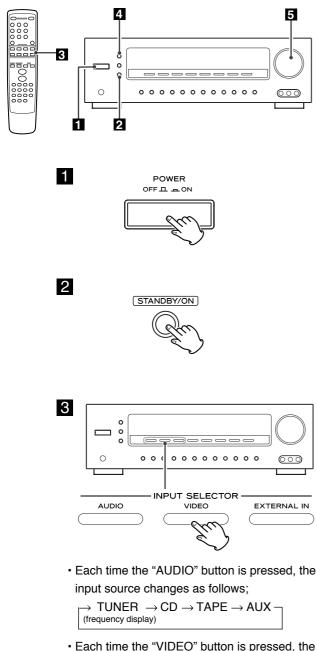
Each time the "VIDEO" button is pressed, the input source changes as follows;
